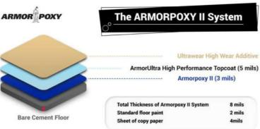
So... Armorpoxy II is over 4 times thicker than floor paint!
